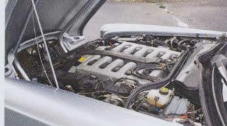
▲ A V12 engine sits under the now front hinged bonnet.
